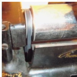
A newly manufactured Neoprene belt for the Edison Fireside. Scoff if you like, but it works!
